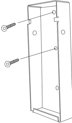
The back piece of the mounting bracket has 3 holes to support attachment to various surfaces. Use the top two holes to attach the mounting bracket to a wall stud.
