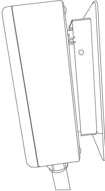
5. Secure the charger in place by inserting either the security pin or the outdoor security lock into the mounting bracket.
