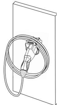
**Note:** Remove rubber cap from charging gun before inserting into holster. Failure to do so may result in damage to the cap or holster.
