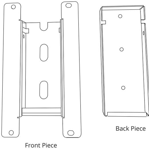
2. Attach the front piece of the mounting bracket to the back of the charging station using the Front Plate screws and hex key tool. Ensure the top of the mounting bracket is matched with the top of the charging station.
